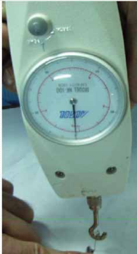
Pic. 1: Set pull meter to zero, ready for testing.
