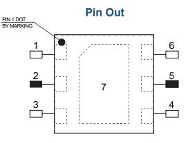
Notes: 1.Require to add Capacitors of DC Blocker between Pins(with black color) and external circuit to prevent DC signal entry to guranteeparts normal work.
